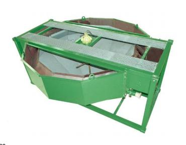
The unit is fitted with an electro-hydraulic power pack with 4kW motor driving a low speed, high torque Staffa motor, which turns a vertical shaft agitator. The agitator is equipped with low and mid level blade assemblies. A fixed ladder provides access to flowforge decking on the upper surface.
